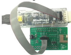
Fig 3: Programming/Debugging with MiniProg3
