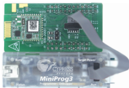
Fig 3: Programming/Debugging with MiniProg3
