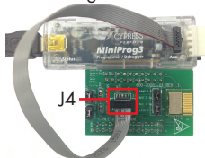
Fig 3: Programming/Debugging with MiniProg3
