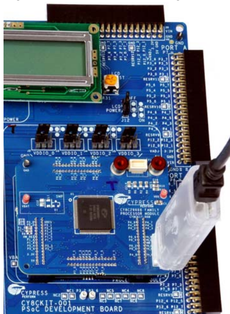
Figure 2-9. Connect MiniProg3 to J5 on CY8C29 Family Processor Module
