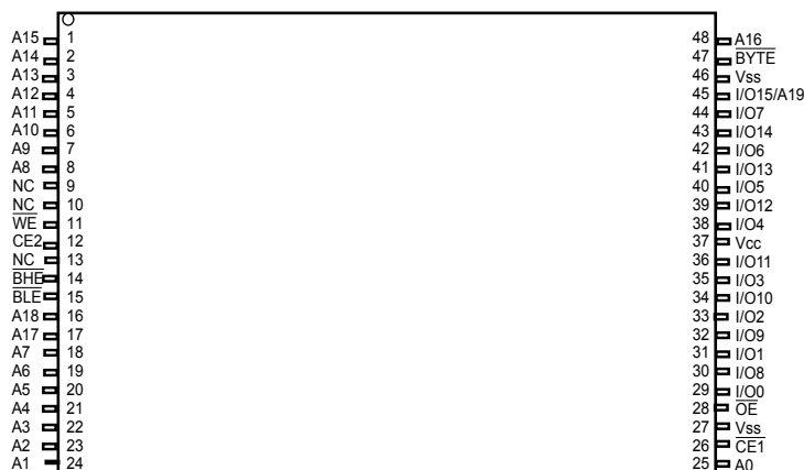
Figure 3. 48-pin TSOP I pinout (Top View) [1, 3]
