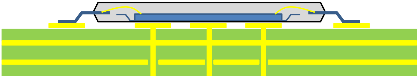
Figure10.2-1: Example thermal via holes on PCB.
