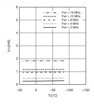
$I_{CCL} - T_A$   $V_{CC} = 5.5 \text{ V}, F_{MPL} = 16 \text{ kHz (divided by 2)}$ Subclock mode with the external clock operating
