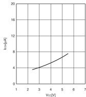
$I_{CCMCR} - V_{CC}$  $T_A = +25^{\circ}C$ ,  $F_{MP} = 4$  MHz (no division) Main CR clock mode
