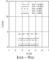
$T_A = +25^{\circ}C$ ,  $F_{MP} = 2, 4, 8, 10, 16$  MHz (divided by 2) Main sleep mode with the external clock operating
