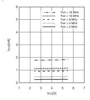
$I_{CCL} - V_{CC}$   $T_A = +25^{\circ}C, \; F_{MPL} = 16 \; kHz \; (divided \; by \; 2)$  Subclock mode with the external clock operating
