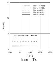
Vcc = 5.5 V, FmP = 2, 4, 8, 10, 16 MHz (divided by 2) Main sleep mode with the external clock operating
