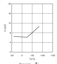
ICCMCR - TA  $V_{CC} = 5.5 \text{ V}, F_{MP} = 4 \text{ MHz (no division)}$
