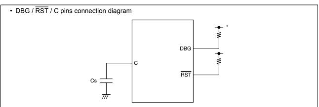
\*: Connect the DBG pin to an external pull-up resistor of  $2 \text{ k}\Omega$  or above. After power-on, ensure that the DBG pin does not stay at "L" level until the reset output is released. The DBG pin becomes a communication pin in debug mode. Since the actual pull-up resistance depends on the tool used and the interconnection length, refer to the tool document when selecting a pull-up resistor.
