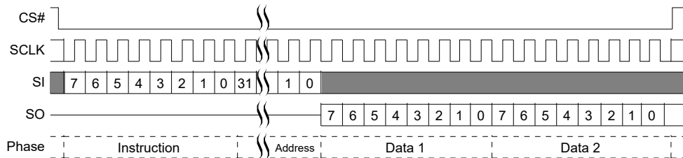
Figure 9. Single Bit Wide I/O Command without latency
