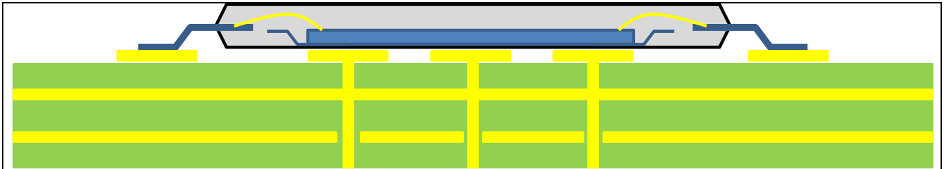
Figure 7-1: Example Thermal Via Holes on PCB.
