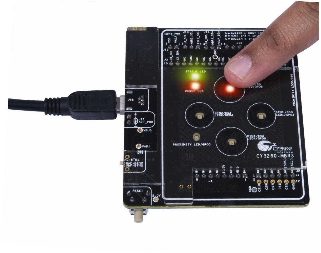
Figure 5-6. Verify LED Toggle Feature
