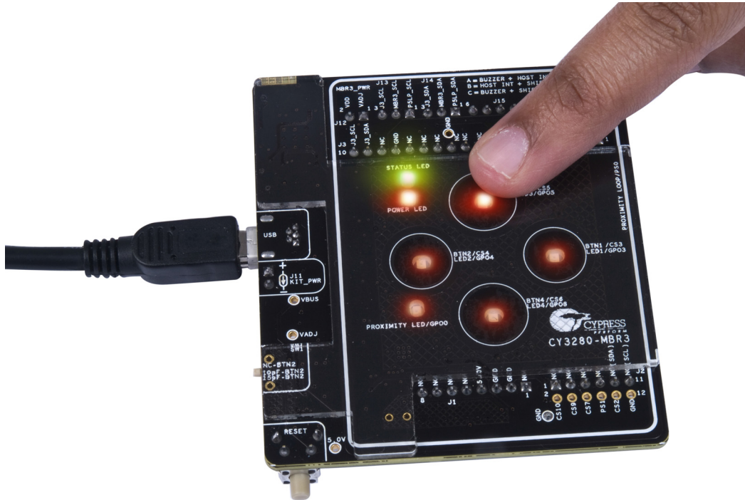
Figure 5-8. LEDs with 93 Percent Brightness on Button Touch
