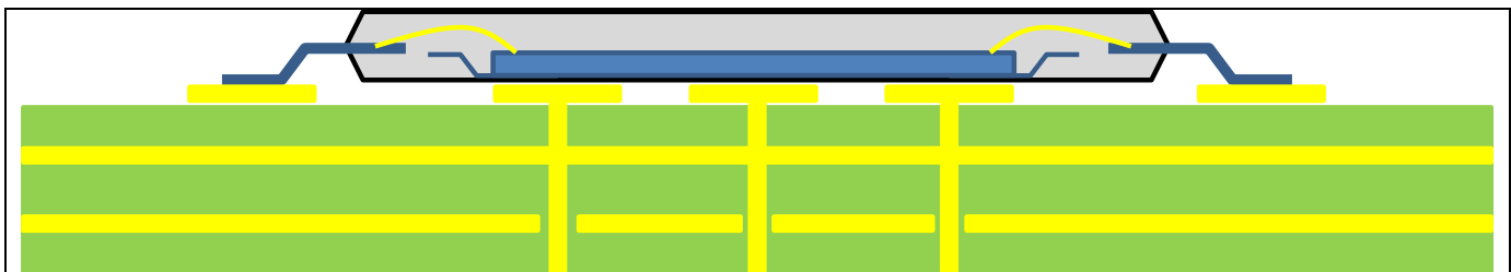
Figure 8-1: Example Thermal via Holes on PCB.
