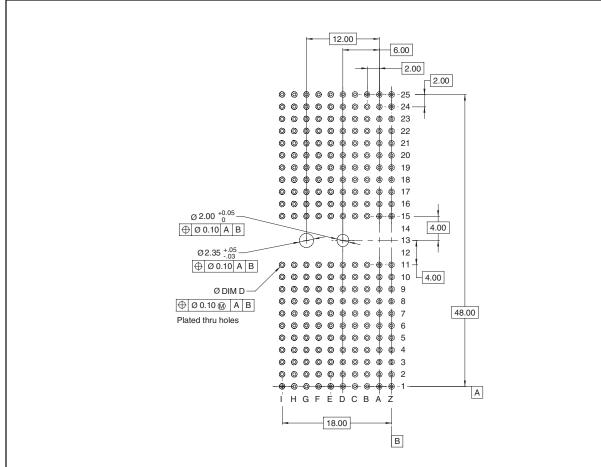
Recommended PCB hole mounting pattern
