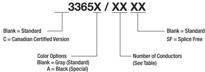
Note: Available in standard 100 ft and 300 ft rolls, please specify when ordering. Contact 3M for availability of additional conductor counts and/or custom roll lengths.
