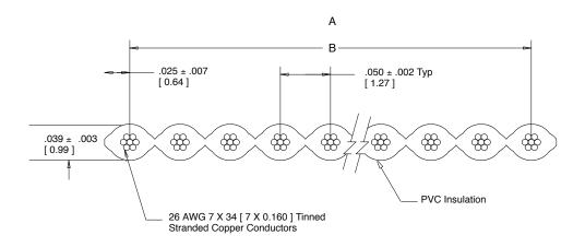
Note: Red marking on one edge of cable designates wire #1.
