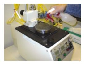
7. Move the fixture in place and lower it gently onto the film, taking care to not gouge the film. The pressure can be experimented with, and may be different from previous polishing steps.
