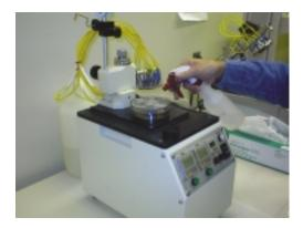
4. Wipe the surface of the 3M<sup>TM</sup> Lapping Film with a clean tissue. The goal here is to remove the air bubbles, smooth out the film and clean the surface of the film. The film should be wiped until almost completely dry and laying flat.
