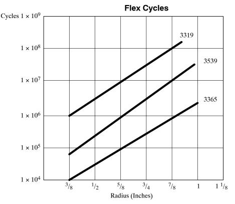
The ability of a cable to withstand repeated flexing without conductor failure is determined by the severity of the flexing (radius of flex) and by the composition and /or constructions of each conductor. The "**Flex Cycles**" chart presents test data comparing three conductor constructions/compositions at various bend radius. The "**Rolling Flex Test**" flexed the cable 180° around a radius closely resembling typical usage, as represented in the illustration below.
