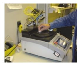
5. This shows the film well adhered to the back-up pad, laying smooth and clean.
