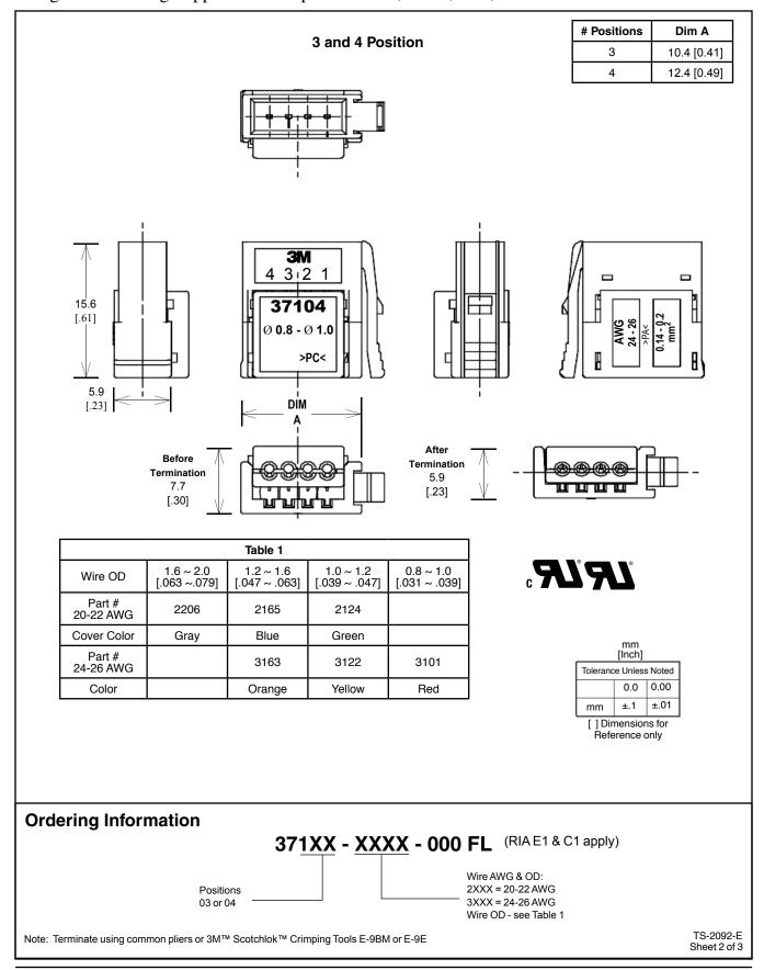
Designed for Wiring Supplied from Japan and Asia, 2 mm, IDC, Wiremount
