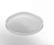
3M™ Bumpon™ Protective Product SJ5382 is a self-adhesive rubber bumper designed to be used as feet, stops and spacers. The hemispherical shape provides excellent sound damping and energy absorption. Clear, 6.4 mm. wide x 1.9 mm. high.
