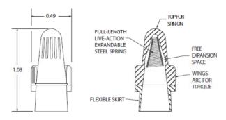
Specifications – Engineering/ Architectural 3M™ Wire Connector O/B+ is capable of connecting two or more wires in a pigtail application, in the wire range of No. 22 thru No. 12 AWG solid and/or stranded copper conductors. The connector shall be constructed with an active (live) spring with a corrosion resistant coating.
