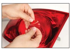
**5.** Press firmly and evenly across all areas of the film to ensure good adhesion and prevent moisture and dirt from entering the lamp.
