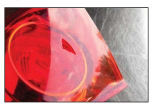
2. The repair film should be cut large enough to overlap the repair by about 1/2 inch on all sides to ensure good adhesion of the film. Hold the repair film up to the damaged area and lightly trace the amount of film needed for the repair with a marker.
