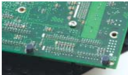
Printed Circuit Board Spacers Fig.101
