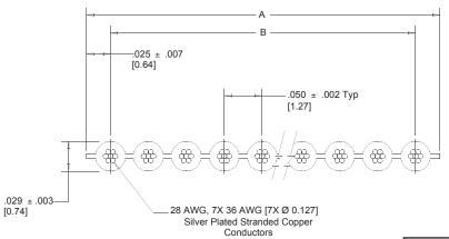
Note: Blue marking on one edge of cable designates wire #1.
