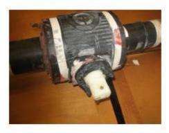
Figure 4-10 Close-up of Valve Operator and Remnants of Actuator Nut
