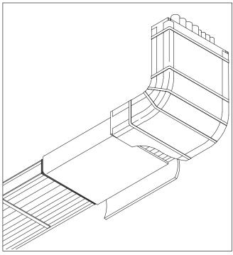
**Figure 7B:** Wrap first layer of E-Mat around the cable tray straight section. Complete the layer with a 2 inch (5 cm) minimum overlap. Secure mat using 3M<sup>™</sup> 898 Filament Tape.
