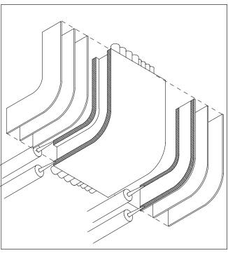
Figure 6B: Cut three pieces of E-Mat for each side of the cable tray. Cut the E-Mat pieces large enough to fit over the cable tray sides and cover edges of inner and outer wrap pieces already installed. Before installing side pieces, apply 3M™ Fire Barrier Sealant CP 25WB+ to inner and outer E-Mat edges as shown. Install sides pieces and secure using 3M™ 898 Filament Tape.
