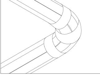
Figure 3D: Apply  $3M^{\text{TM}}$  425 Sealing Tape over all exposed seams and caulk.
