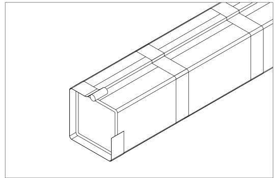
3 - Repeat these steps for all subsequent layers as per listing/design. A new stainless steel band is to be installed at the termination after the final end cap layer has been installed.
