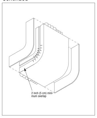
**Figure 5E:** Cut and install the third side layer of 3M<sup>™</sup> Interam<sup>™</sup> Systems E-Mat as shown. Secure mat using 3M<sup>™</sup> 898 Filament Tape.
