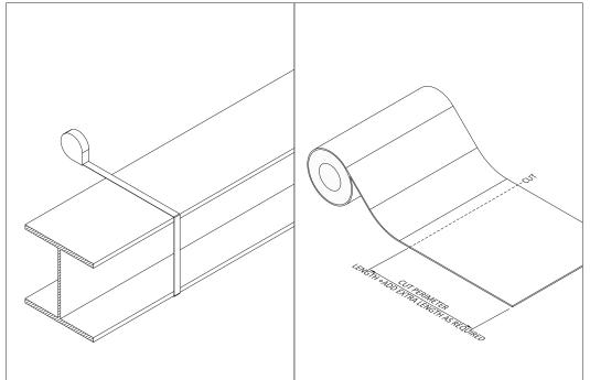
2 - Cut Endothermic Mat 5A-4 (EMat) to length using bladed edge. Align EMat to the steel with foil side facing outward (white side should be in contact with steel). Edge of EMat can be held in place by filament tape or by other worker. Wrap EMat around the steel then overlap itself by a minimum of 2 inches (50 mm) (Figure 3). Additional overlap is acceptable but not required. EMat should be tight to the steel, free of slack.
