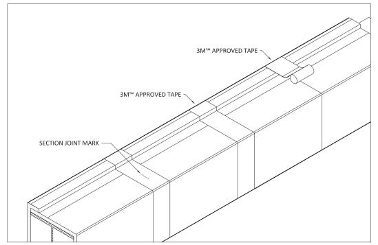
6 - If additional layers are required, measure the perimeter of the first layer and add additional length to accommodate for overlap and corner bending. Stagger the perimeter joints of the second layer by minimum of 2 inches (50 mm) away from the perimeter joints in the first layer. The reference points are used to ensure the 2 inch stagger distance. Repeat steps 1 through 5 (Figure 7)
