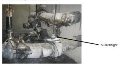
Figure 4-12 Specimen C Following Hose Stream Test
