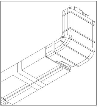
Figure 7F: Apply 3M<sup>™</sup> 425 Sealing Tape over all mat edges and seams.
