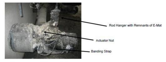
Figure 4-8 Specimen A Following Hose Stream Test
