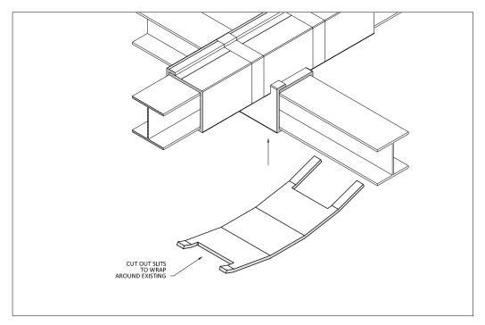
3 - Repeat step 1 and 2 for all subsequent layers as per listing/design, alternating between wrapping the top and bottom sections. Once the last layer of EMat is in place, secure the EMat with stainless steel banding. (Refer to Chapter 1 for specifications surrounding stainless steel banding). The final layer where the EMat interfaces between the bottom and the top beam should be caulked by approved 3M caulking to prevent moisture from penetrating the joint.
