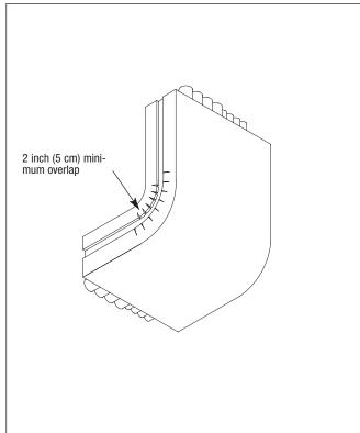
**Figure 5D:** Apply top and bottom E-Mat pieces as shown and secure using  $3M^{\text{TM}}$  898 Filament Tape.
