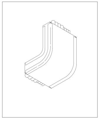
**Figure 5F:** Apply 3M<sup>™</sup> 425 Sealing Tape to all E-Mat seams.
