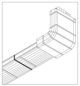
**Figure 7A:** Install  $3M^{TM}$  Interam<sup>TM</sup> Systems E-Mat to cable tray elbow sections following steps 5A to 5G or steps 6A to 6D.
