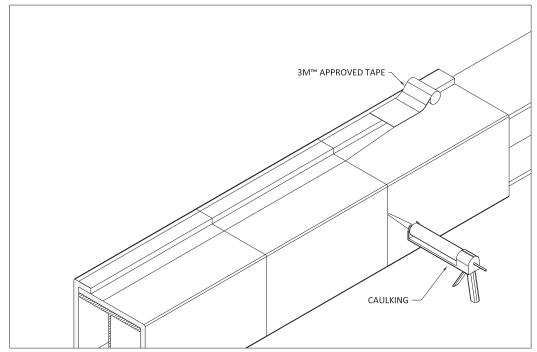
5 - The butt seam where the two pieces meet (perimeter joint) is to be covered with 3M approved tape. Tape and then mark the location of the joints on the tape using a soft tipped marker to establish a reference point. Smooth the tape with a hard roller or straight edge applying enough pressure to ensure adequate adhesion of the tape to the EMat and to remove any air gaps (Figure 6).
