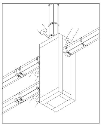
**Figure 4D:** Apply 3M<sup>™</sup> 425 Sealing Tape over all exposed mat seams and caulked edges. Apply 3M<sup>™</sup> Fire Barrier Sealant CP 25WB+ around interface between wrapped conduit and box as shown.
