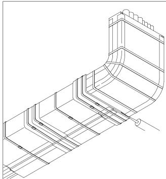
**Figure 7H:** Apply  $3M^{TM}$  Fire Barrier Sealant CP 25WB+ to fill any gaps between the collar and the E-Mat sections underneath it. Apply steel banding within 2 inches (5 cm) of each collar edge, and at 12 inches (30 cm) maximum throughout the system.
