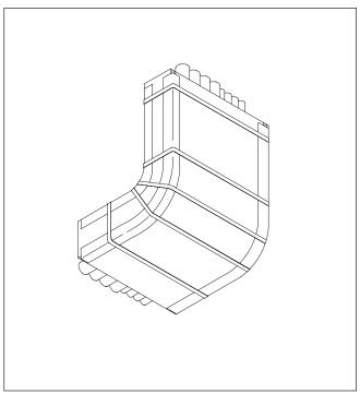
Figure 6D: Install steel banding around the cable tray every 12 inches (30 cm) maximum and within 2 inches (5 cm) of each cable tray end. See Figures 7A to 7H for details regarding a transition of the cable tray elbow to a cable tray straight section.
