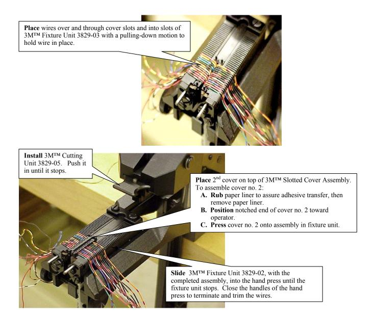
Completed Assembly of the Two Covers and Cable
