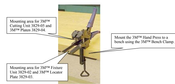
Cover set-up and installation
