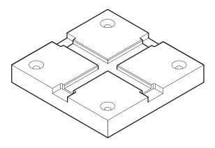
Note: This locator plate can only be used with press platen 3442-9, which must be ordered separately.
