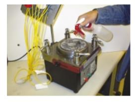
4. Wipe the surface of the 3M<sup>TM</sup> Lapping Film with a clean tissue. The goal here is to remove the air bubbles, smooth out the film and clean the surface of the film. The film should be wiped until almost completely dry and laying flat. This photo shows the film well adhered to the back-up pad, laying smooth and clean.
