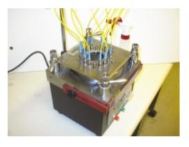
After the cycle, carefully lift the fixture, to minimize scoring of the film. The film can be wiped dry, and placed in an area for the next use.
