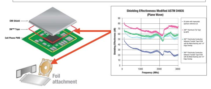
3M<sup>TM</sup> Electrically Conductive Adhesive Transfer Tapes 9703, 9404, 9705, 9706, 9708, 9709, 9709S, 9709SL, 9712, 9713, 9714 and 7805 can provide FPC grounding and tapes 9708, 9709, 9709S, 9709SL and 7805 can increase the effective EMI Shielding through the bond line thickness leading to improved product EMI Shielding performance of the FPC.
