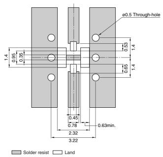
Line width be designed to mach  $50\Omega$  characteristic impedance depending on PCB material and thickness
