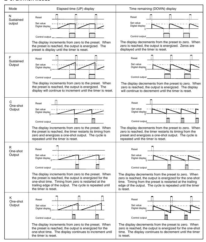
**NOTE:** In modes F and K, when the 99 min 59 s or 99 h 59 min ranges are selected in DOWN display, the overflow values will be shown as 9959, 9958, 9957, etc.
