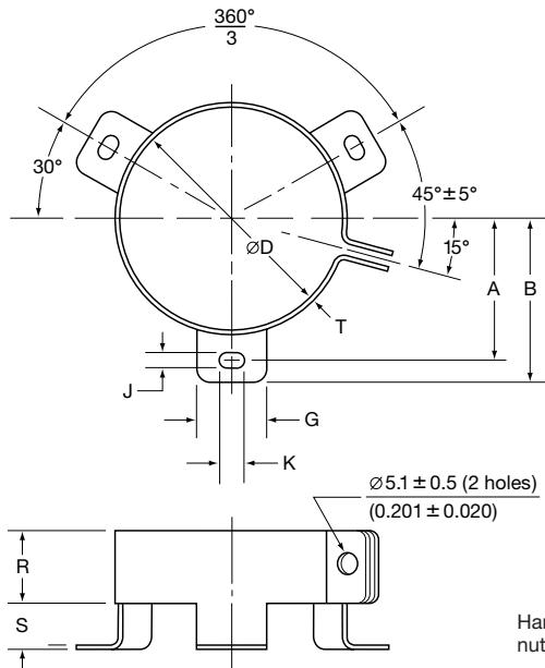
Hardware: Screw, washer and hexagon nut included with each clamp.
