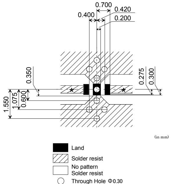
\* Line width to be designed to match 50 ohm characteristic impedance,
