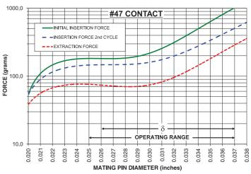
**The insertion / extraction force characteristics above** were derived using a 30 microinch gold-plated contact and polished steel gauge pins having a bullet-shaped tip. The curves represent typical average values; they are best used to compare the differences between similar size contacts and to guide you in selecting one that is suitable for your application. Your results may vary, so for your specification, we encourage you to obtain complimentary samples for your evaluation.
