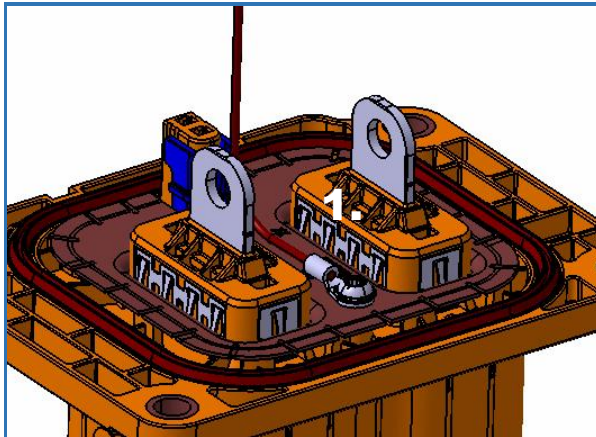
Fig. 4.16: Fitting the annular ring attachment 2way
