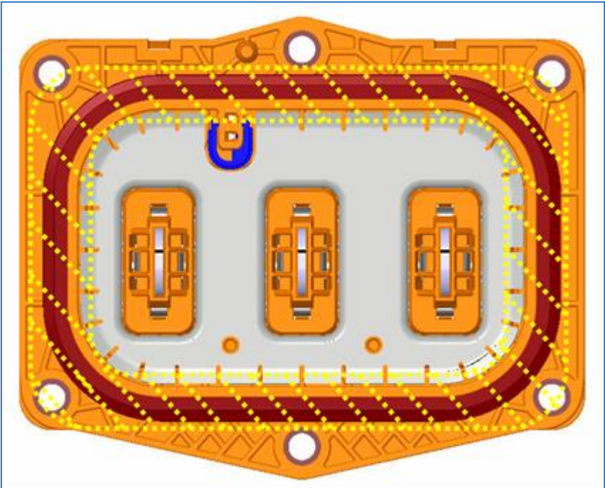
Fig. 7.5: Sealing area of the 3 way KHV 600 tab header
