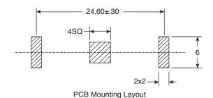
**SPECIFICATIONS** Material: 0.25mm Phosphor Bronze Nickel Plated **Battery Size:** CR2032 **RoHS Compliant**
