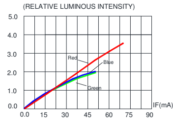
FIG.2 RELATIVE LUMINOUS INTENSITY VS. FORWARD CURRENT
