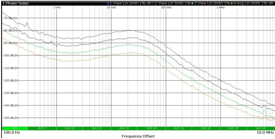
Figure 30 Phase noise plot of 3.2GHz RF PLL, I_{cp}=400\mu A , F_{Comp}=19.2MHz , using internal VCO, 60kHz loop bandwidth, PLL type ‘1100’ also showing output in /2 mode (1600MHz), /4 mode (800MHz) and /8 mode (400MHz)
