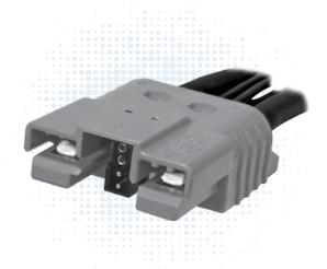
SBE® and SBO® connectors build on the capability of the two pole SB® connectors by offering up to 8 auxiliary power / signal contacts along with an IEC 60950 touch safe housing. The center of the main connector features a connector holder for either: two PP15-45, two PPMX, or APP's innovative 1x4 auxiliary connector.
