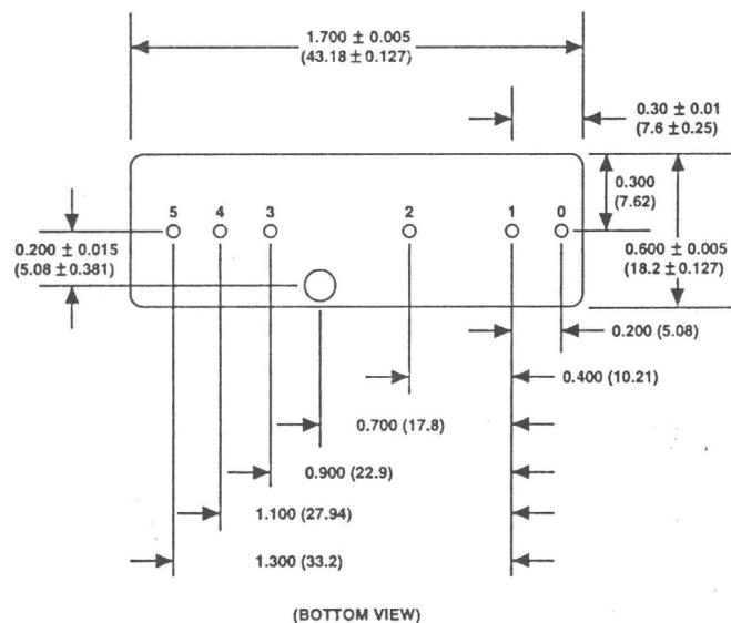
Figure 4 . Model 7B Series Module, with pin-out assignments.
