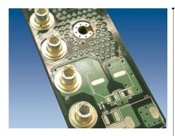
RADSERT™'s compact footprint design can deliver up to 120A of current to the board. The high current density and small surface area connection provides flexibility of board design. RADSERT™ contacts are available in either press-fit or solder termination.
