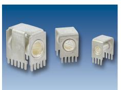
The RADSOK® PGY™ provides a compact and robust right angle power to board interconnect. Designed to mate with either a 3.6mm or 5.7mm pin, The RADSOK® PGY™ can bring up to 120A to the board. The radial design of the RADSOK® contact gives you more contact surface area lowering temperature rise and reducing potential heat related failures.
