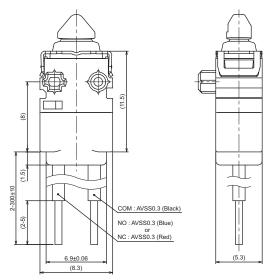
**Note:** UL approved wires (AWG24, UL1007) are used for UL/cUL standard approved items.
