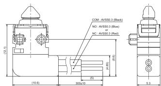
**Note:** UL approved wires (AWG24, UL1007) are used for UL/cUL standard approved items.
