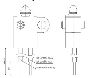
**Note:** UL approved wires (AWG24, UL1007) are used for UL/cUL standard approved items.
