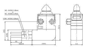
**Note:** UL approved wires (AWG24, UL1007) are used for UL/cUL standard approved items.
