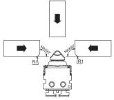
**Note:** Do not operate from the direction shown in the figure below. It is not designed to be operated from this direction.
