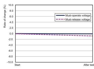
Characteristics are measured after vibration at the frequency of 33Hz,  $45\text{m/s}^2$  is applied to the test piece (not energized) in vertical direction for 4 hours and in each left, right, front and back directions for 2 hours.
