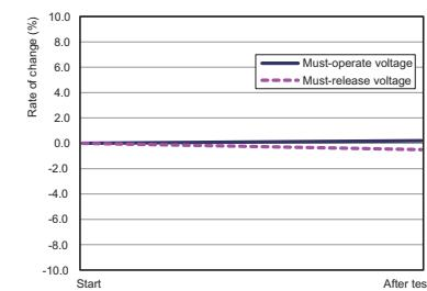
Characteristics are measured after vibration at the frequency of 33Hz, 45m/s<sup>2</sup> is applied to the test piece (not energized) in vertical direction for 4 hours and in each left, right, front and back directions for 2 hours.
