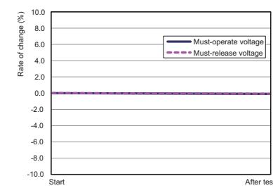
Characteristics were measured after applying a shock of 490 m/s<sup>2</sup> to the test piece 3 times each in 6 directions along 3 axes. The percentage rate of change is the average value for all of the samples.
