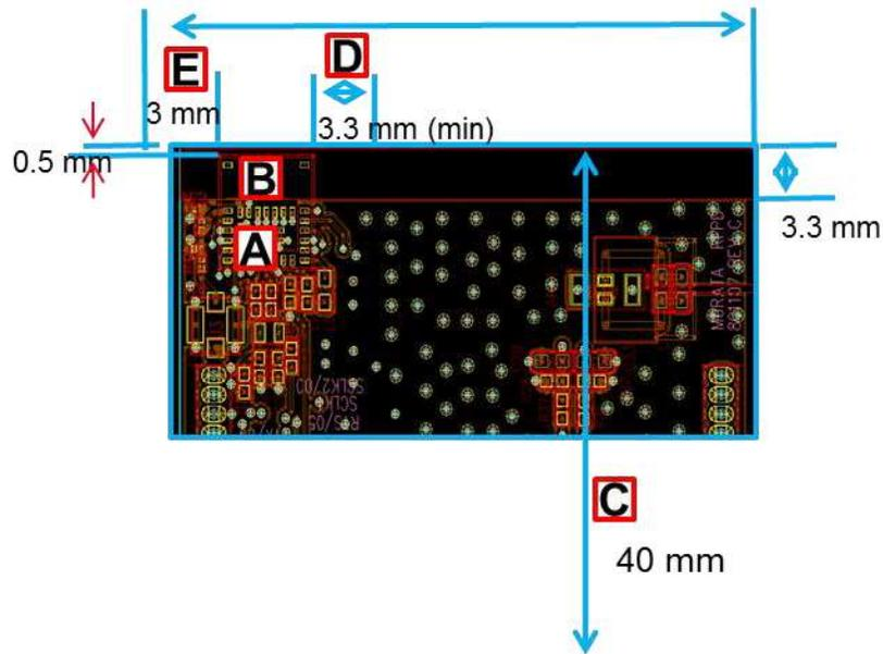
**Figure 7.3 Layout Guide for Antenna Performance (1)**
