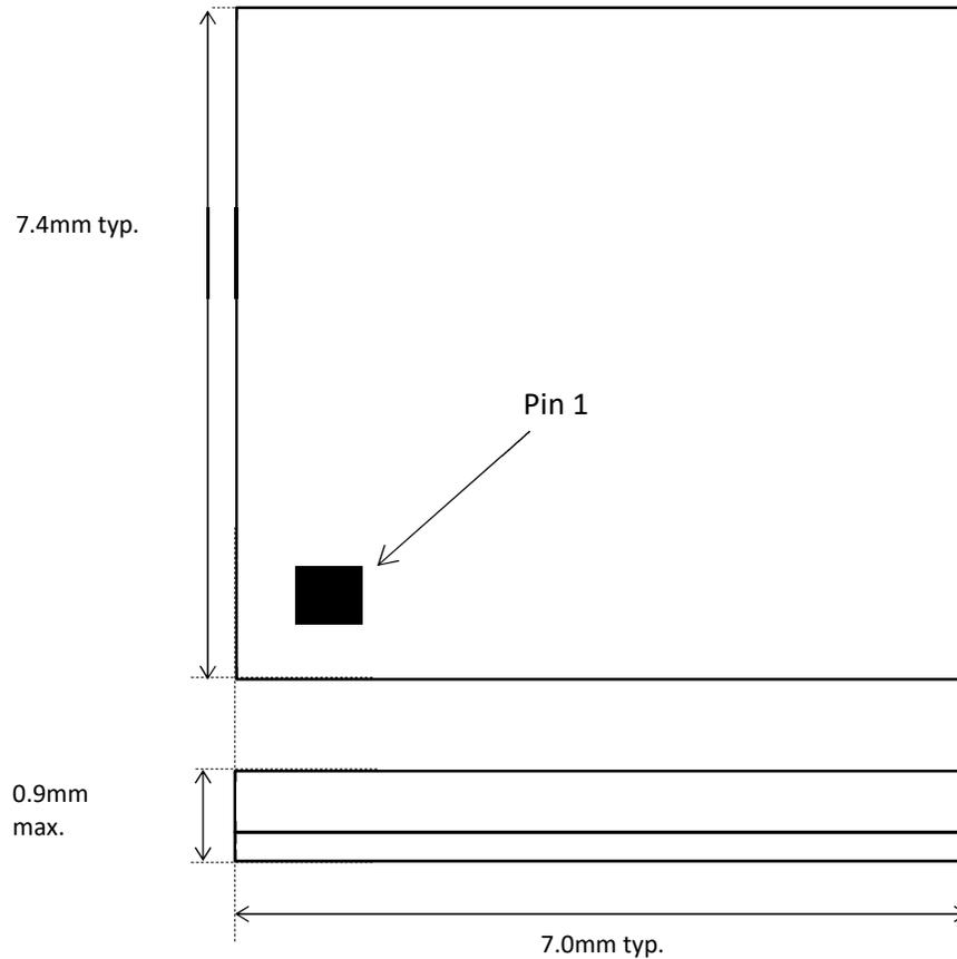
Figure 2.1 Module Top and Side View (Unit: mm)
