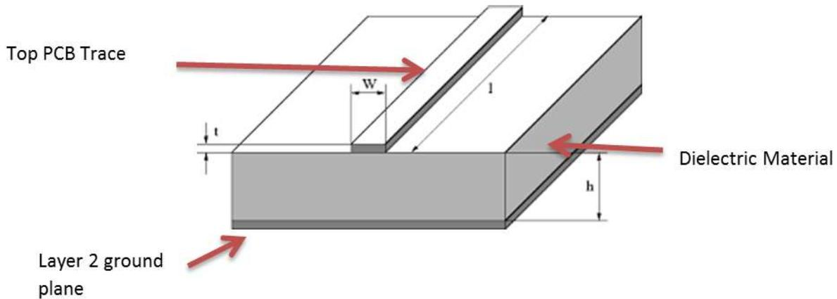
**Figure 7.6 Layout Guide for External Antenna (2)**
