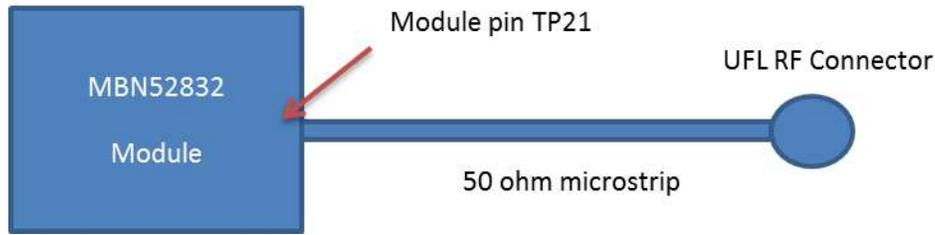
**Figure 7.5 Layout Guide for External Antenna (1)**
