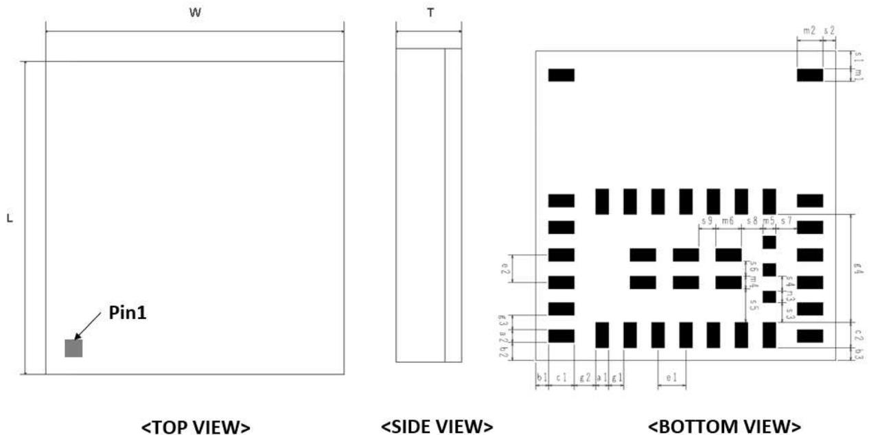
Figure 2.2 Module Footprint Top View (Unit: mm)
