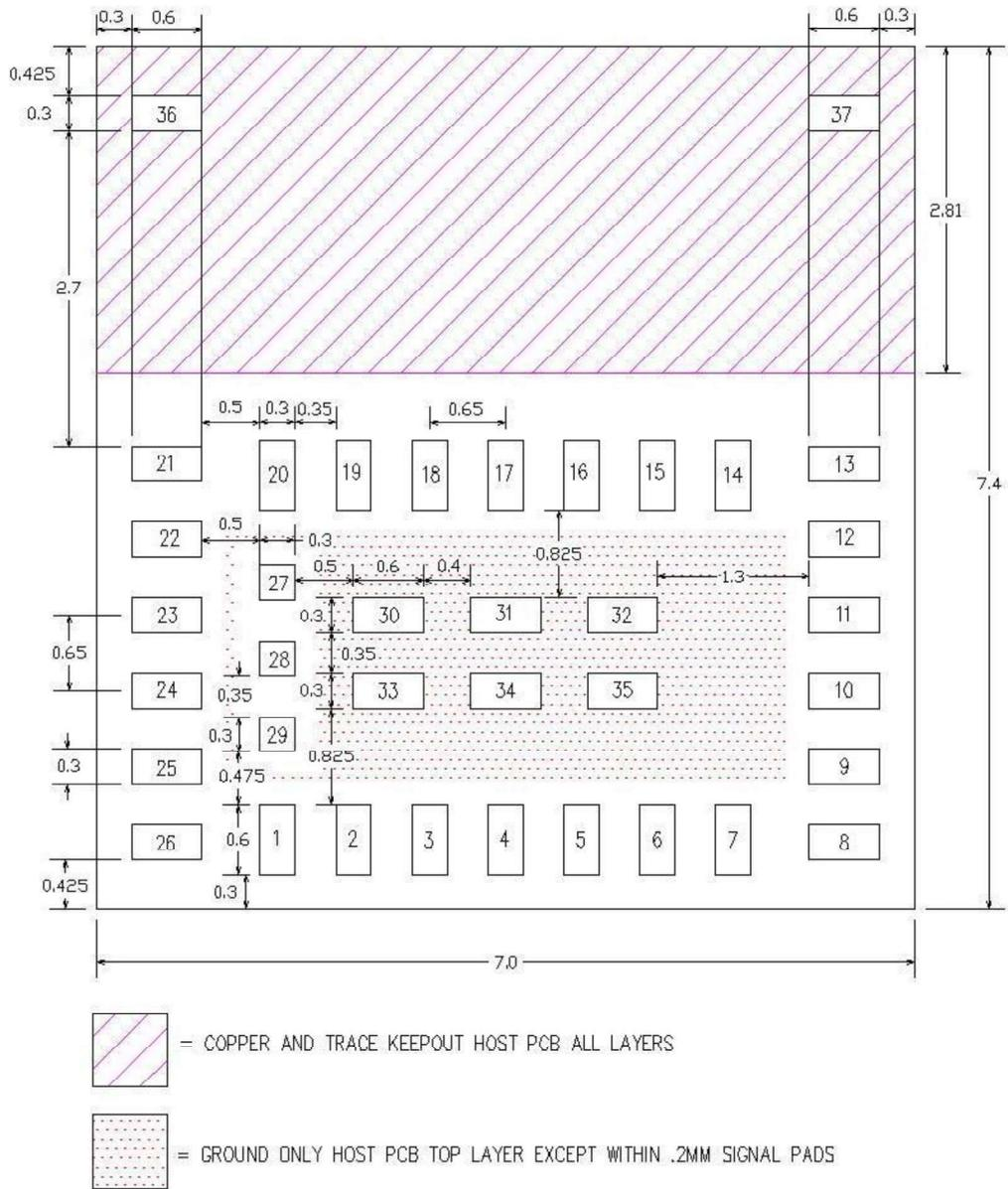
**Figure 7.2 Host PCB Layout Recommendation, top view**
