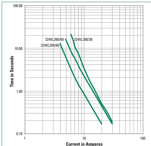
Note: The average time current curves and Temperature Derating curve performance is affected by a number of variables, and these curves provided as guidance only. Customer must verify the performance in their application.
