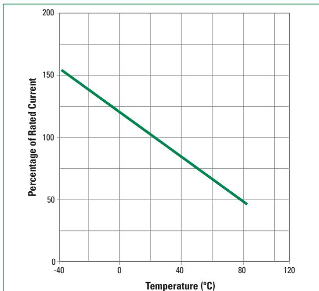
Note: Typical Temperature derating curve, refer to table for derating data.
