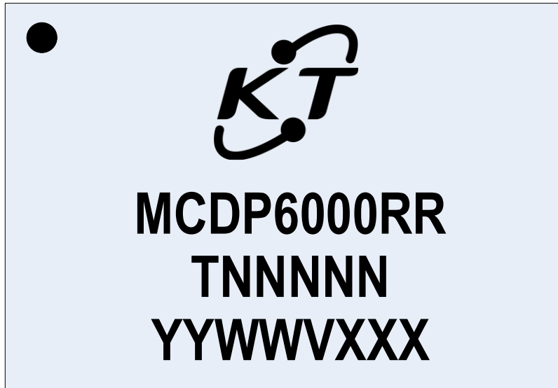
Figure 15. MCDP6000 Ex-VQFN46 Marking Template
