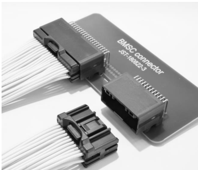
0.64 terminal, 2.2 mm pitch dual-row, board-to-wire connector for automotive applications.
