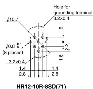
Remarks : Dimensional tolerance of  $\pm 0.05$ mm is recommended for the board arrangement.
