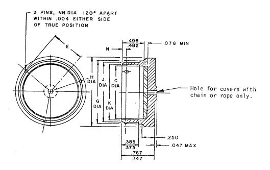
FIGURE 2. Protective cover, plug, bayonet coupling M83723/59-2.
