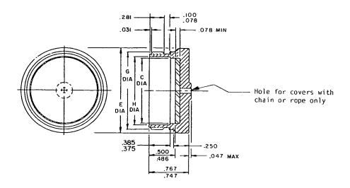
FIGURE 1. Protective cover, plug, threaded coupling M83723/59-1.
