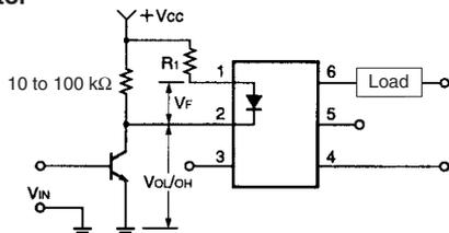
Use the following formula to obtain the LED current limiting resistance value to assure that the relay operates accurately.
